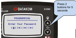
A 4 digit password must be entered using buttons.
